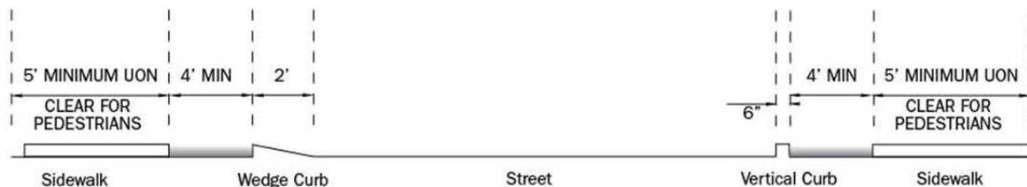
**Figure 4 - TYPICAL CROSS SECTION**
